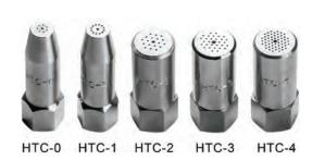
$\rm HTC$  series tips are the same as the HT series except they have center orifices, which allow a better range when used with high pressure natural gas.
